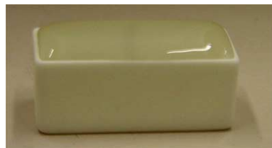
Fig. 4. Rectangular boat used for water transpiration tests with different amounts of water in the boat. Because of the various amounts of water the height of the rim varies. The picture shows the boat filled with 19 g of water. The water surface layer exceeds the height of the sidewalls by about 0.1 cm.
